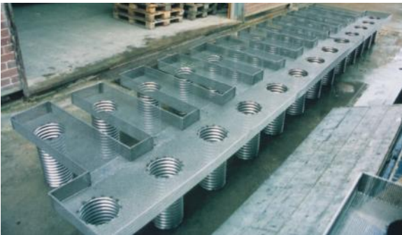
Special casing for machine foundation
